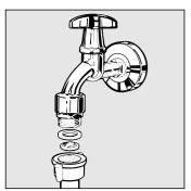
This hose is **not** suitable for use for connection to a hot water supply. Please make sure that the washer sits correctly in the union.
